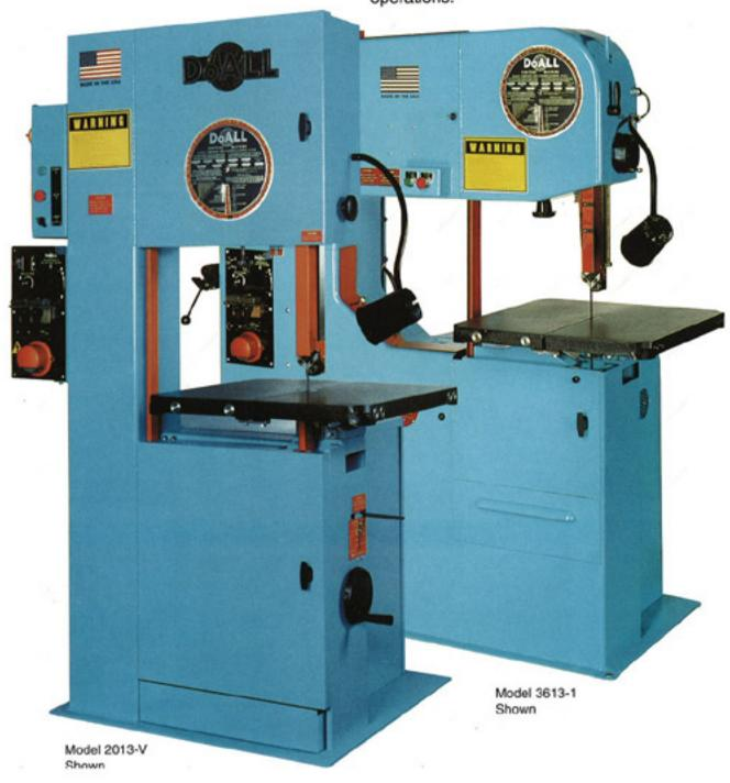
All four models have a 26" x 26" table that tilts 45" right and 10" left plus feature a 13" maximum workheight to handle a wide variety of material sizes. A variable speed drive and 2 speed transmission permit you to choose the optimum band speed when cutting different materials. And, you can use saw blades from 1/16" to 1" width.
