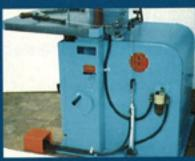
Optional welder (left) welds coil blade stock to length and allows for internal cuts.
